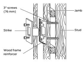
Furnished with standard and round corner deadbolt strikes, this reinforcer significantly strengthens a jamb against "kick-in" attack and greatly increases the security of the lock. The reinforcer is concealed under the strike and is anchored to the jamb with two 3" long screws. B500 Series metal dust box reinforcer anchors (B520-622) to jamb with three 3" screws.
