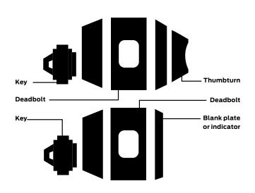
Standard cylinder. FSIC - full size interchangeable core option. SFIC - small format interchangeable core option. Complies with ADA Accessibility Guidelines.
