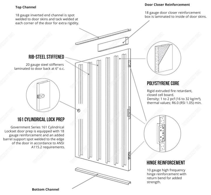
18 gauge inverted end channel is spot welded at each corner of the door for extra rigidity.
