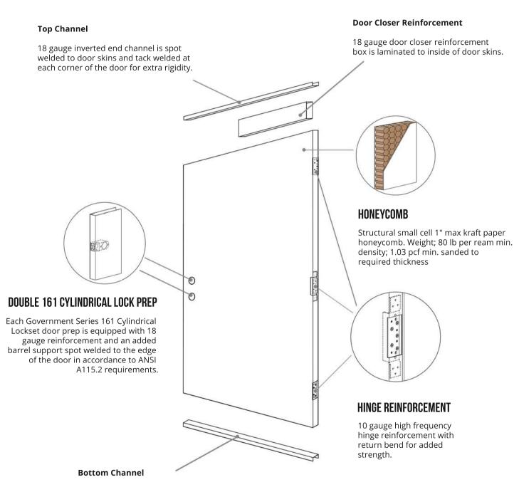
18 gauge inverted end channel is spot welded at each corner of the door for extra rigidity.
